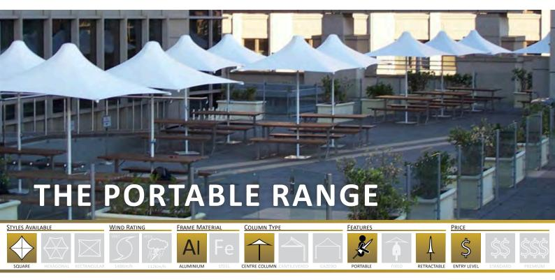
Our Portable range is designed to be light & easy to handle, easily removable from inground sockets or above-ground base plates, compatible with a large assortment of existing tables and sockets, yet able to withstand wind gusts of up to 60 kph
