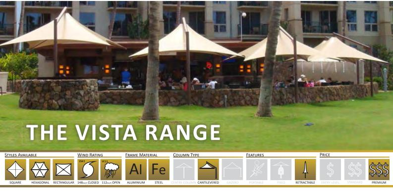
The Vista range has a cantilevered frame ideal for pools, cafes and public spaces where clear space under the canopy is preferred. The optional 360 degree pivoting base is perfect for utilising the shade at varying times of the day or for covering more than one area.
